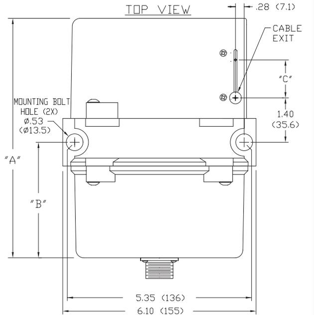
ON MODELS WITH ZERO AND SPAN CONTROLS, REMOVE SELF SEALING SCREWS TO ACCESS ADJUSTMENT POTENTIOMETERS.
